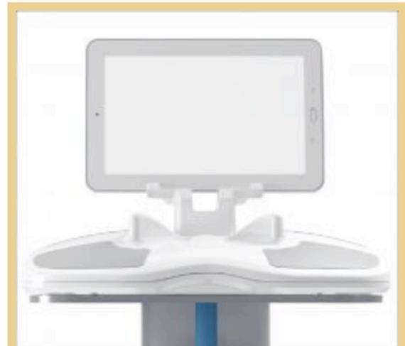
The digital health platform technology uses L-Dex measurements, which are made by passing a harmless electrical signal of very low strength from the device through the patient's limbs. (Credit: Impedimed)
